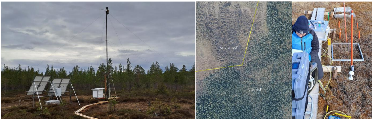
Fig. 10. Left) The eddy covariance measurement set-up for measuring \text{CO}_2 flux at Matorovansuo peatland. Middle) Drained and undrained source areas of the EC measurement. Data are attributed according to wind direction. Right) Chamber measurements were conducted in trenched and intact, vegetated points. The peatland type is a pine flark fen. Photos Jack Chapman, satellite image from National Land Survey of Finland 2023.
